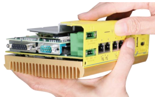
Install I/O panel
